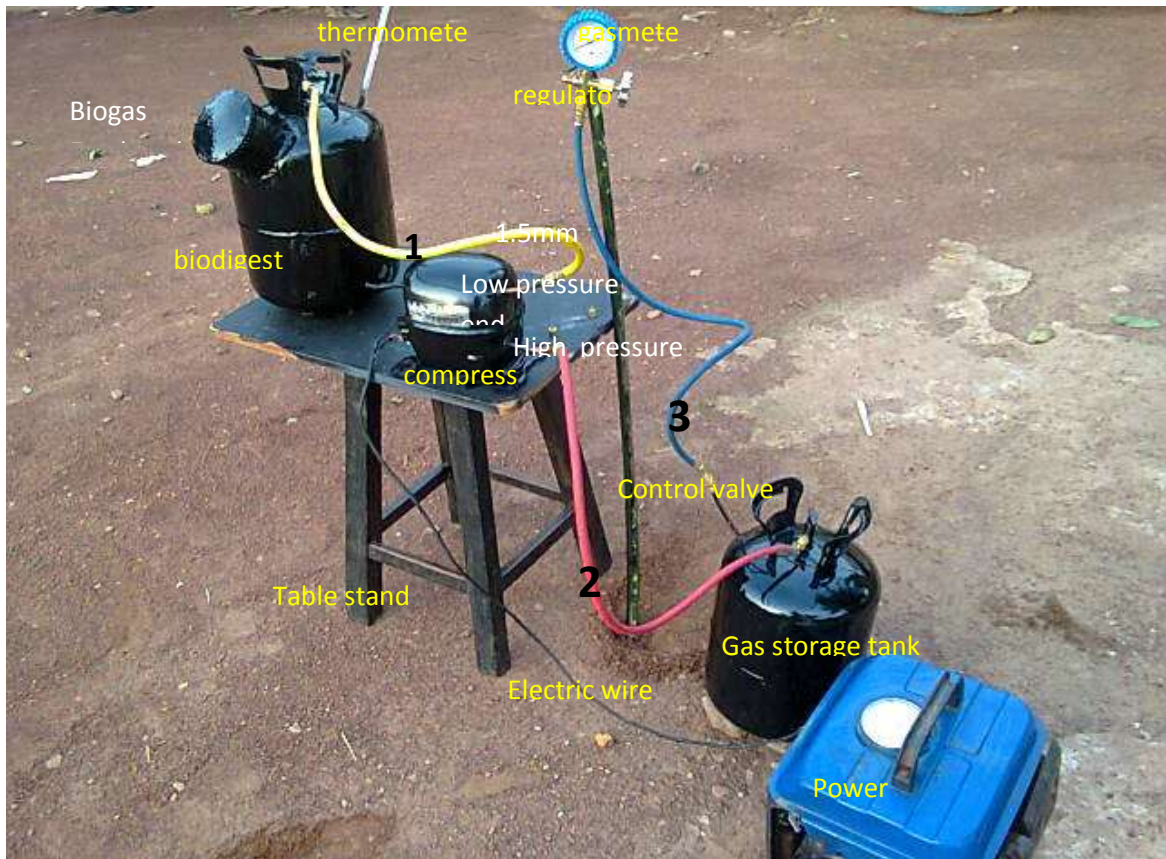
Figure 1: Biogas Production Pilot Plant Assembly (plant)
